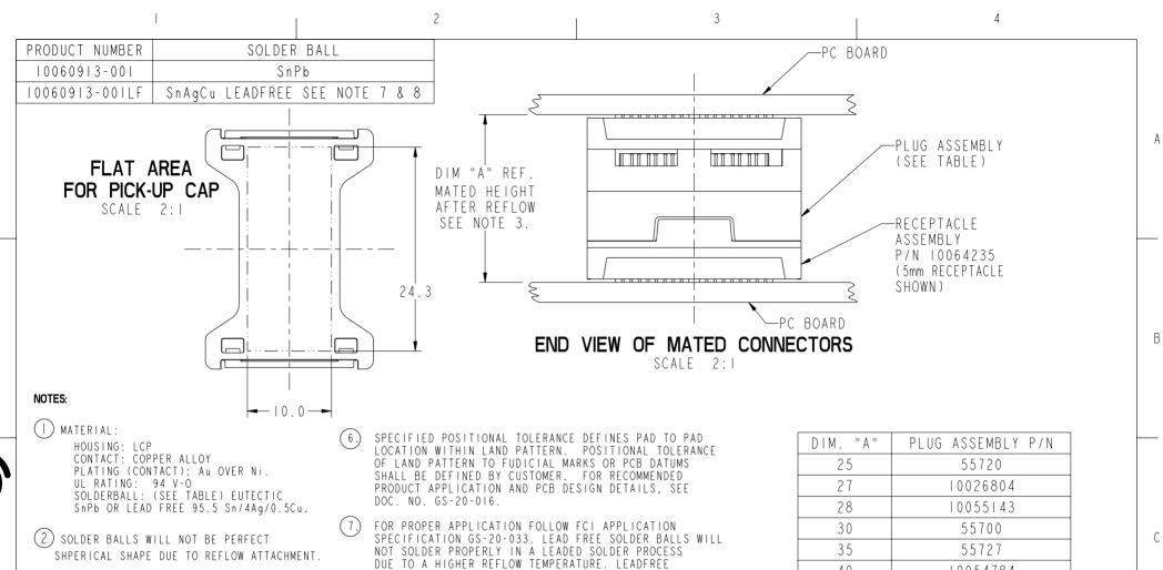
(3) mated height effected by customers? PCB PAD SIZE, PLATING, SOLDER REFLOW PROFILE & SOLDER PASTÉ.
